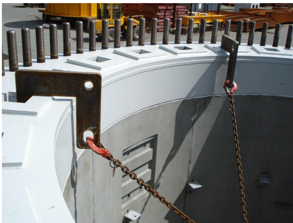
Figure 6: Example for fixation tooling for the connection-element during the transport
