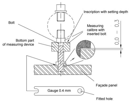
KEIL undercut anchor KH for facade panels Corian EC,
