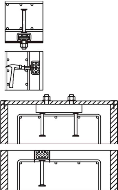
**a) Fixing to steel formwork**
