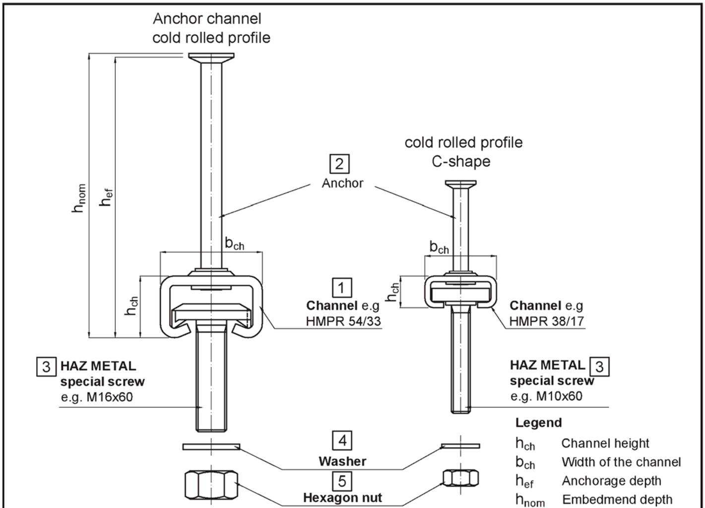
**Marking of the HAZ - anchor channel :
