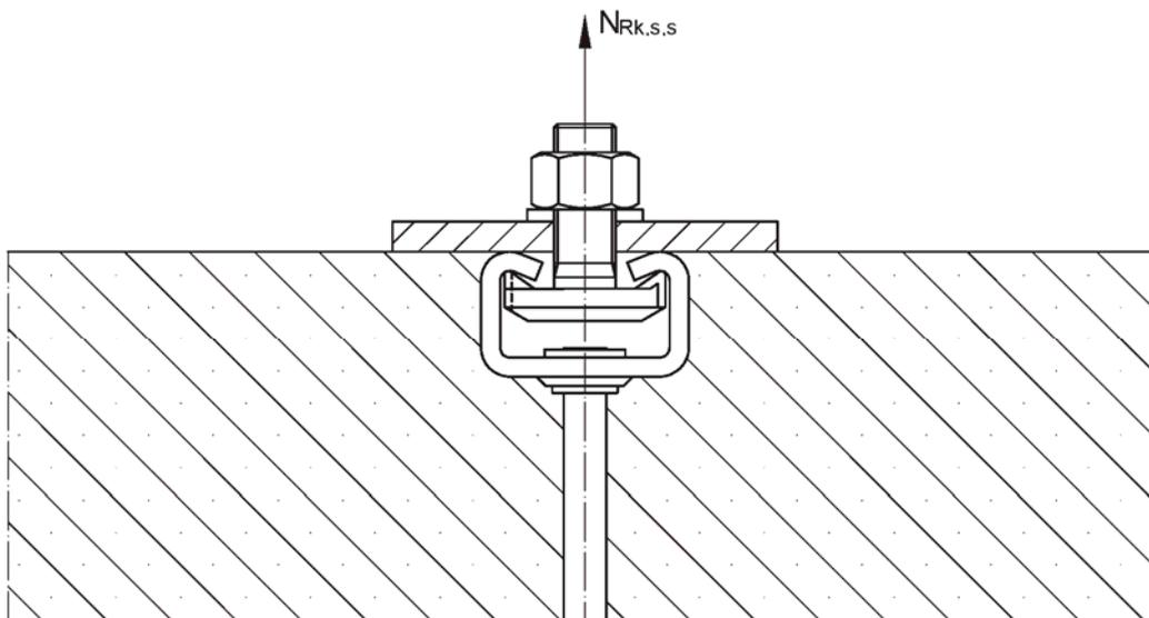
Channel under tension load
