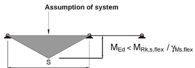
Table 10: Flexure resistance of channel
