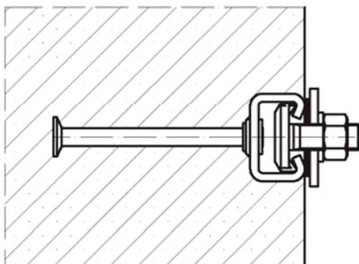
1. Use washers between the channel and the fixture to create a defined contact.
