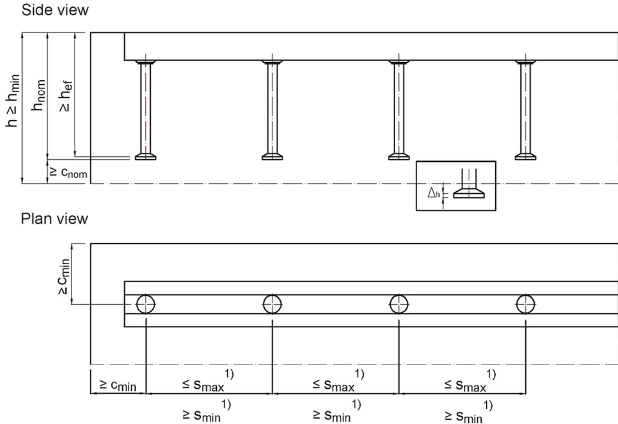
Table 7: Minimum anchorage depth, edge distance and member thickness for cold rolled profiles
