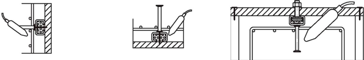
a) sidefaces to the formwork    or    b) in soffits    or    c) into top surfaces of concrete up stands
