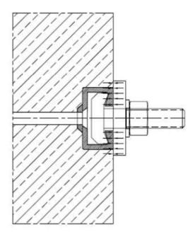
The fixture is braced to the concrete **or** to the anchor channel respectively braced to the concrete **and** to the anchor channel. The setting torque T<sub>inst</sub> according to Table 7, shall be applied and must not be exceeded.
