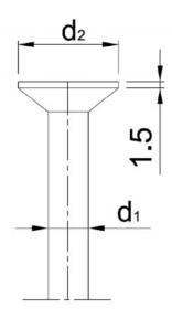
Fig. 4: Anchor for Ski assembled version (cross-section)
