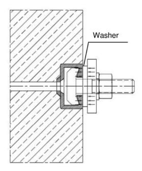
The fixture is braced to the anchor channel by a suitable washer. The setting torque T<sub>inst</sub> according to Table 7, shall be applied and must not be exceeded.
