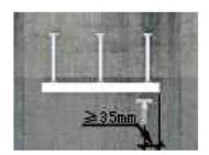
Positioning of the special screw: at the channel ends a minimum clearance must be maintained (≥ 35mm)
