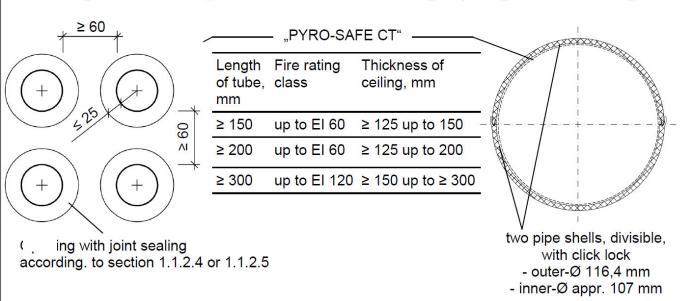
Single or cluster arrangement of Cable-Tubes "PYRO-SAFE CT" in case of one common opening in massif ceilings.
