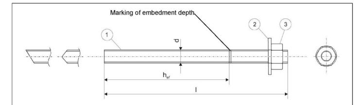
Commercial standard threaded rod M8, M10, M12, M16, M20, M24, M27 or M30 with
