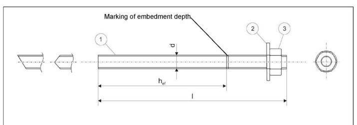
Commercial standard threaded rod M8, M10, M12, M16, M20, M24, M27 or M30 with
