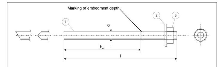
Commercial standard threaded rod M8, M10, M12, M16, M20, M24, M27 or M30 with
