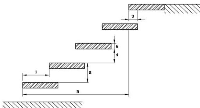
**KENNGOTT - Cantilever step stair**
