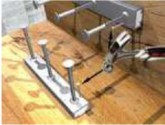
Fixing of the anchor channel to timber formwork with nails through the prefabricated holes in the back of the anchor channel
