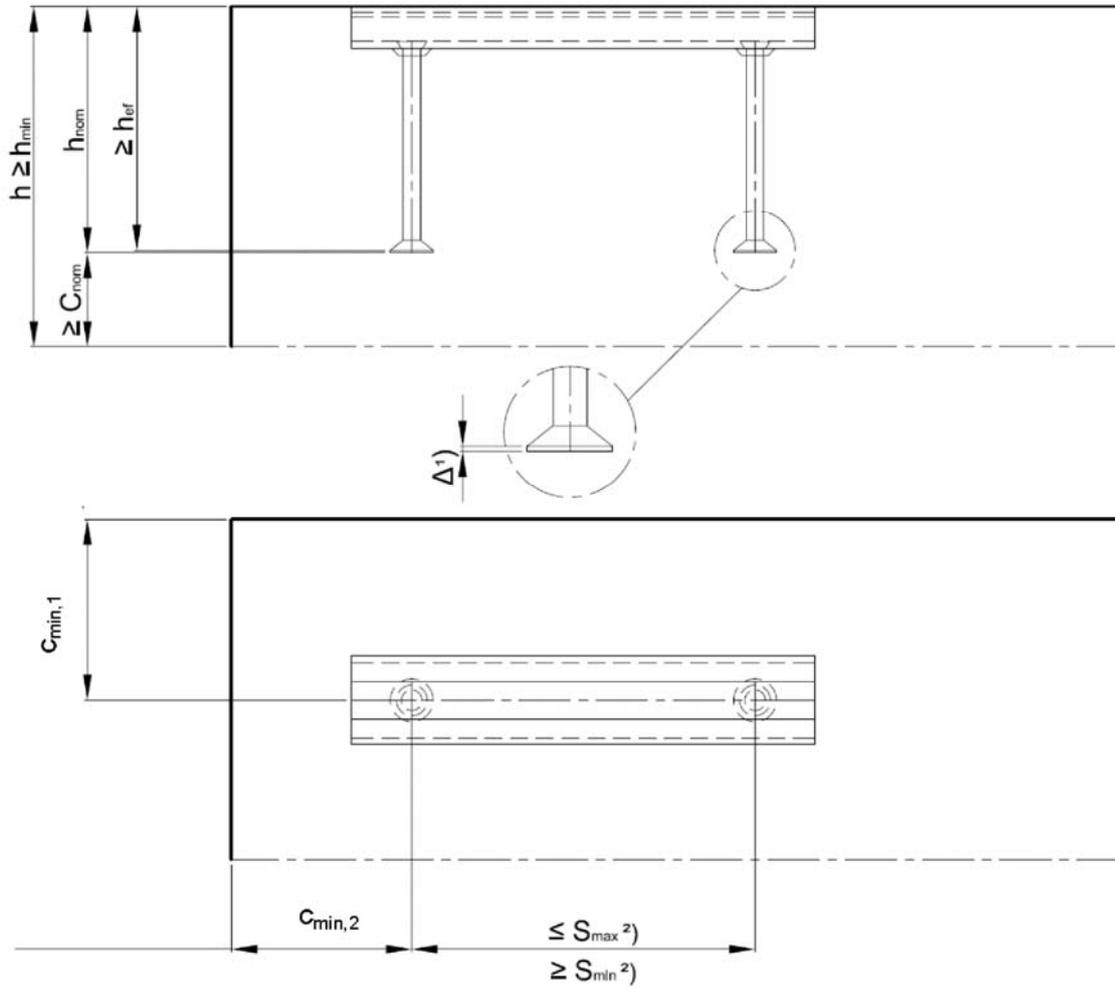
Table 6: Minimum effective anchorage depth, edge distances and member thicknesses
