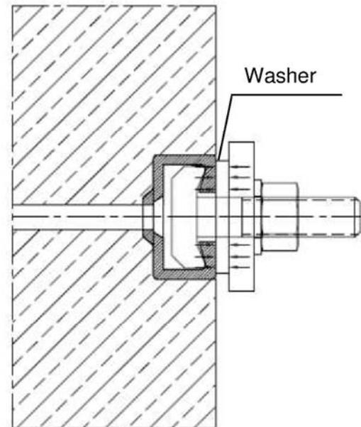
The fixture is braced to the anchor channel by a suitable washer. The setting torque  $T_{inst}$  according to Table 7, shall be applied and must not be exceeded.
