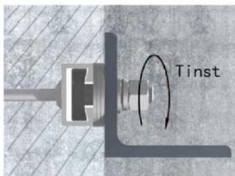
If the anchor channel is embedded below the concrete surface, use washers. ( $T_{inst} = 200\text{Nm}$ )
