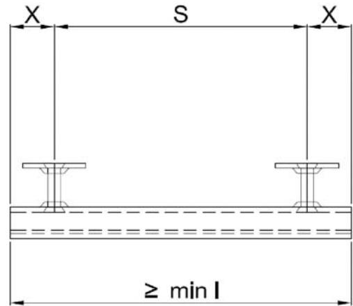
Table 3: Minimum and maximum spacing, end distance and minimum channel length
