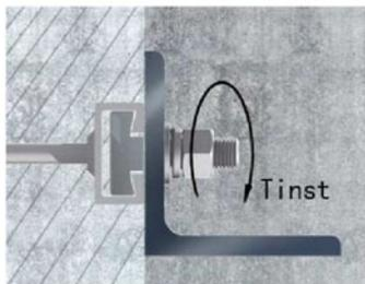
Tighten the hexagonal nut to the setting torque  $T_{inst}$ .
