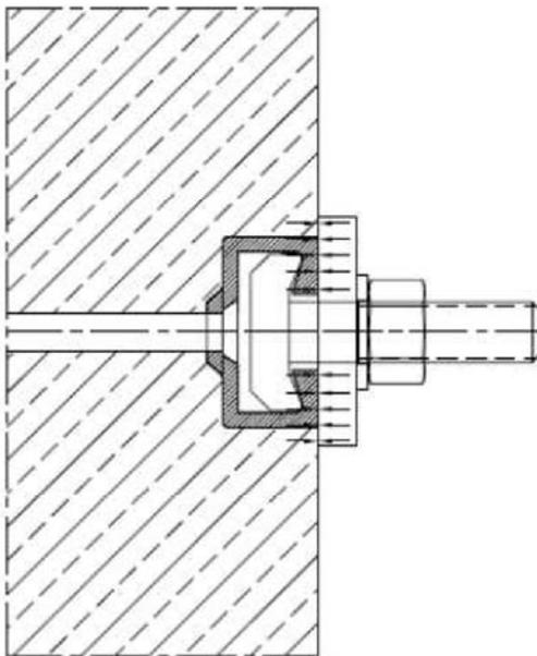
The fixture is braced to the concrete **or** to the anchor channel respectively braced to the concrete **and** to the anchor channel. The setting torque  $T_{inst}$  according to Table 7, shall be applied and must not be exceeded.
