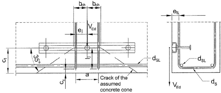
$$V_{Ed} \leq V_{Rd,re} = V_{Rk,re} / \gamma_{Mc} \quad V_{Ed} = \max[V_{Ed}; V_{Ed}^a] \quad (1)$$
