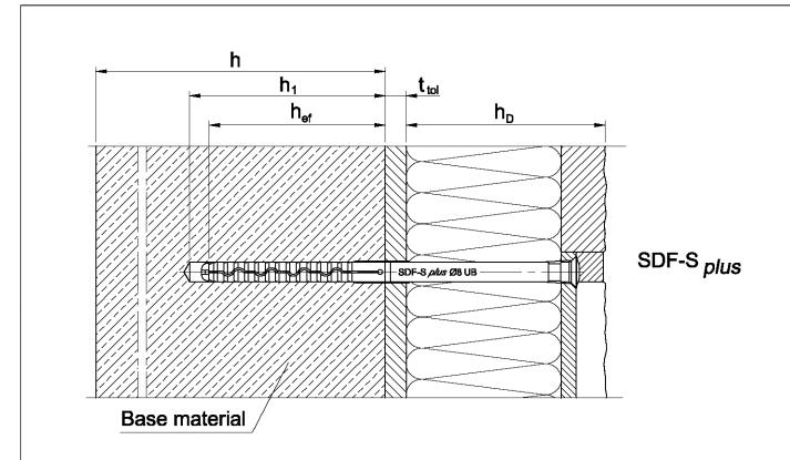
Legend:  $h_D$  = thickness of insulation material
