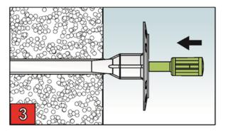
Insert the anchor into the hole until the plate rests on the insulation. hammer in the nail with a matching hammer
