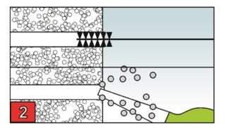
Holes to be cleaned of drilling dust.
