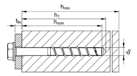
$d_0 \\$ nominal drill bit diamter nominal anchorage depth  $h_{\text{nom}}$ depth of the drill hole  $h_1$
