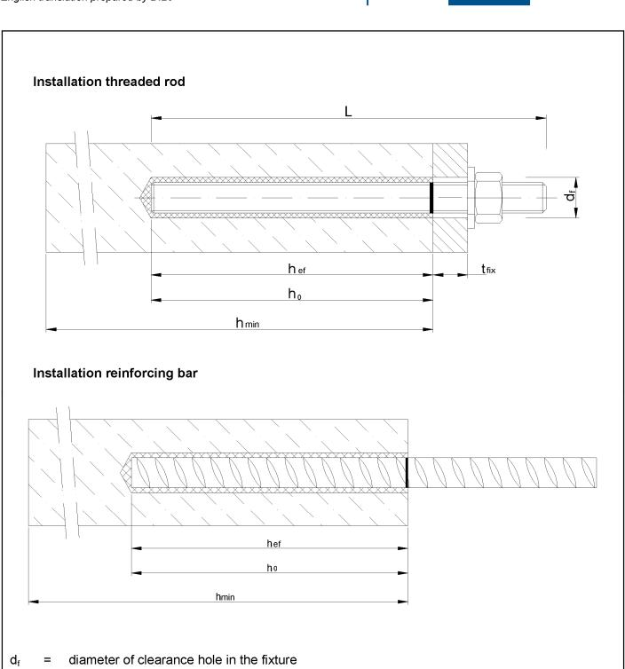
$t_{fix}$  = thickness of fixture
