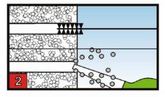
Holes to be cleaned of drilling dust.
