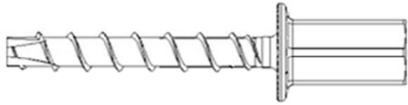
Two circle marks with  $d = 0,8 \text{ mm}$  for  $h_{nom} = 55 \text{ mm}$
