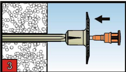
Insert the anchor into the hole until the plate rests on the insulation.
