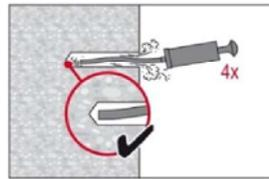
The Hilti manual pump may be used for blowing out drill holes up to diameters  $d_0 \leq 18$  mm and embedment depths up to  $h_{ef} \leq 10 \cdot d$ . Blow out at least 4 times from the back of the drilled hole until return air stream is free of noticeable dust
