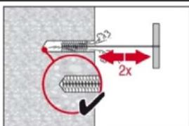
Brush 2 times with the specified brush (see Table B3) by inserting the steel brush Hilti HIT-RB to the back of the hole (if needed with extension) in a twisting motion and removing it. The brush must produce natural resistance as it enters the drilled hole (brush  $\varnothing \geq$  drill hole  $\varnothing$ ) - if not the brush is too small and must be replaced with the proper brush diameter.
