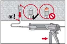
For overhead installation the injection is only possible with the aid of extensions and piston plugs. Assemble HIT-RE-M mixer, extension(s) and appropriately sized piston plug (see Table B3). Insert piston plug to back of the hole and inject adhesive. During injection the piston plug will be naturally extruded out of the drill hole by the adhesive pressure.
