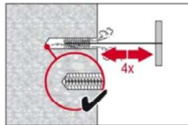
Brush 4 times with the specified brush (see Table B3) by inserting the steel brush Hilti HIT-RB to the back of the hole (if needed with extension) in a twisting motion and removing it. The brush must produce natural resistance as it enters the drilled hole (brush  $\varnothing \geq$  drill hole  $\varnothing$ ) - if not the brush is too small and must be replaced with the proper brush diameter.
