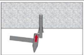
For overhead installation use piston plugs and fix embedded parts with e.g. wedges (Hilti HIT-OHW).
