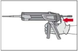
After injection is completed, depressurize the dispenser by pressing the release trigger. This will prevent further adhesive discharge from the mixer.
