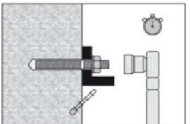
Loading the anchor: After required curing time  $t_{cure}$  (see Table B2) the anchor can be loaded.
