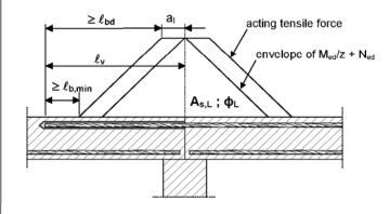
Figure A4: Rebar connection for components stressed primarily in compression.
