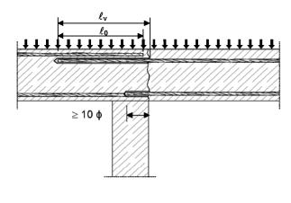
**Figure A2:** Overlap joint with existing reinforcement at a foundation of a column or wall where the rebars are stressed in tension
