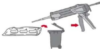
Discard initial mortar. The foil pack opens automatically as dispensing is initiated. Depending on the size of the foil pack an initial amount of mortar has to be discarded.
