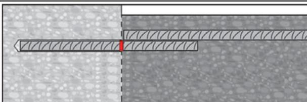
Full load may be applied only after the curing time " $t_{cure}$ " has elapsed (see Table B3)
