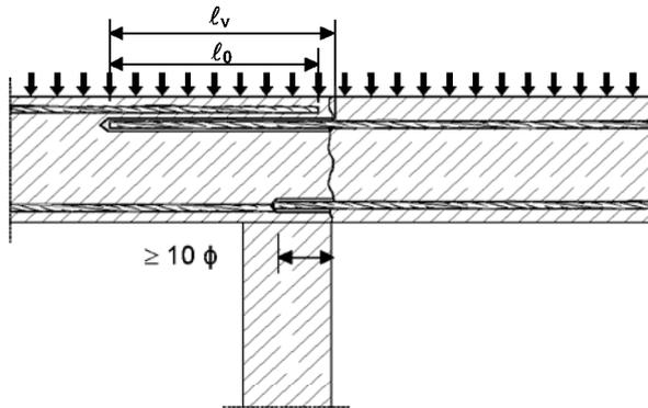
**Figure A2:** Overlap joint with existing reinforcement at a foundation of a column or wall where the rebars are stressed in tension
