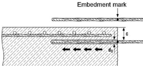
Before use, make sure the rebar is dry and free of oil or other residue.
