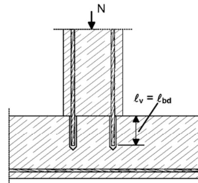
**Figure A5:** Anchoring of reinforcement to cover the enveloped line of acting tensile force in the bending member
