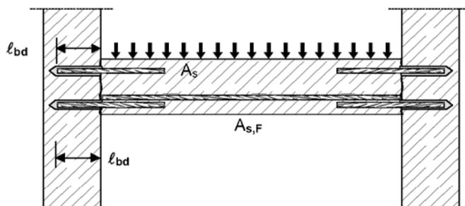
**Figure A4:** Rebar connection for components stressed primarily in compression.
