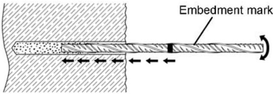
For ease installation insert the rebar slowly twisted into the borehole until the embedment mark is at the concrete surface level.
