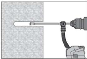
Drill hole to the required embedment depth with an appropriately sized Hilti TE-CD or TE-YD hollow drill bit with Hilti vacuum attachment.
