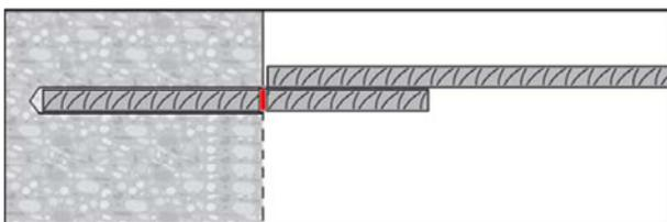
Observe the working time " $t_{work}$ ", which varies according to temperature of base material. Minor adjustments of the rebar position may be performed during the working time.
