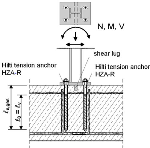
**Figure A7:** Overlap joint for the anchorage of barrier posts
