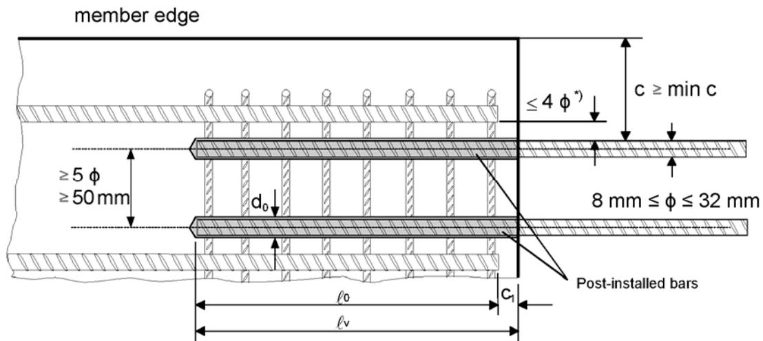
⁹) If the clear distance between lapped bars exceeds  $4 \phi$ , then the lap length shall be increased by the difference between the clear bar distance and  $4 \phi$ .
