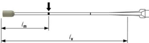
Mark the required mortar level  $l_m$  and embedment depth  $l_b$  resp.  $l_{e,ges}$  with tape or marker on the injection extension.
