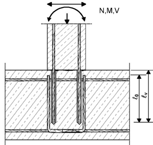
**Figure A3:** End anchoring of slabs or beams
