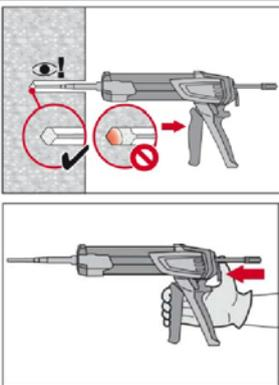
Inject the mortar from the back of the hole towards the front and slowly withdraw the mixing nozzle step by step after each trigger pull.
