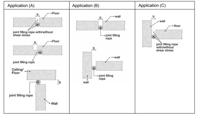
For the number of layers and the arrangement of the joint filling rope, see Table B.2 and B.3.
