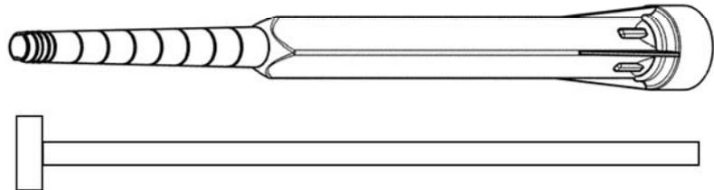
**Betonstahl (rebar):  $\varnothing 8, \varnothing 10, \varnothing 12, \varnothing 14, \varnothing 16, \varnothing 20, \varnothing 22, \varnothing 24, \varnothing 25$**
