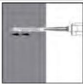
6. Starting from the bottom or back of the cleaned anchor hole fill the hole up to approximately two-thirds with adhesive. Slowly withdraw the static mixing nozzle as the hole fills to avoid creating air pockets. For embedment larger than 190 mm an extension nozzle shall be used. For overhead and horizontal installation in bore holes larger than  $\varnothing 20$  mm a piston plug and extension nozzle (Annex B 5) shall be used. Observe the gel-/ working times given in Table B3.
