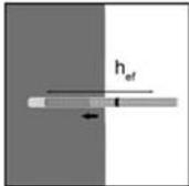
7. Push the threaded rod or reinforcing bar into the anchor hole while turning slightly to ensure positive distribution of the adhesive until the embedment depth is reached. The anchor should be free of dirt, grease, oil or other foreign material.
