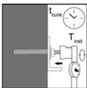
10. After full curing, the add-on part can be installed with the max. torque (Table B1) by using a calibrated torque wrench.
