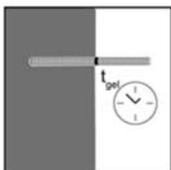
9. Allow the adhesive to cure to the specified time prior to applying any load or torque. Do not move or load the anchor until it is fully cured (attend Table B3).
