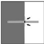
8. Be sure that the anchor is fully seated at the bottom of the hole and that excess mortar is visible at the top of the hole. If these requirements are not maintained, the application has to be renewed. For overhead application the anchor rod should be fixed (e.g. wedges).
