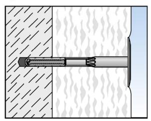
4. Correctly installed anchor
