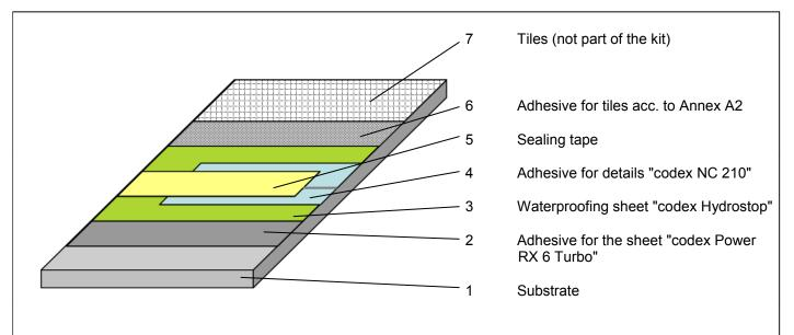
Minimum layer thickness of the waterproofing sheet 0.57 mm
