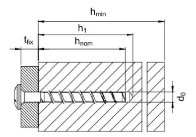
$\begin{array}{lll} d_0 & = & \text{nominal drill bit diamter} \\ h_{\text{nom}} & = & \text{nominal anchorage depth} \\ h_1 & = & \text{depth of the drill hole} \end{array}$
