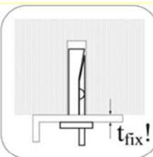
Insert anchor with fixture.
