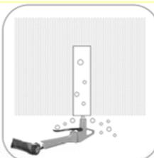
Blow out dust from drilling hole.
