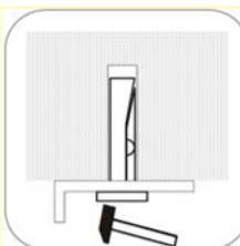
Hammer down wedge. The anchor is properly set if the wedge is fully dropped in.
