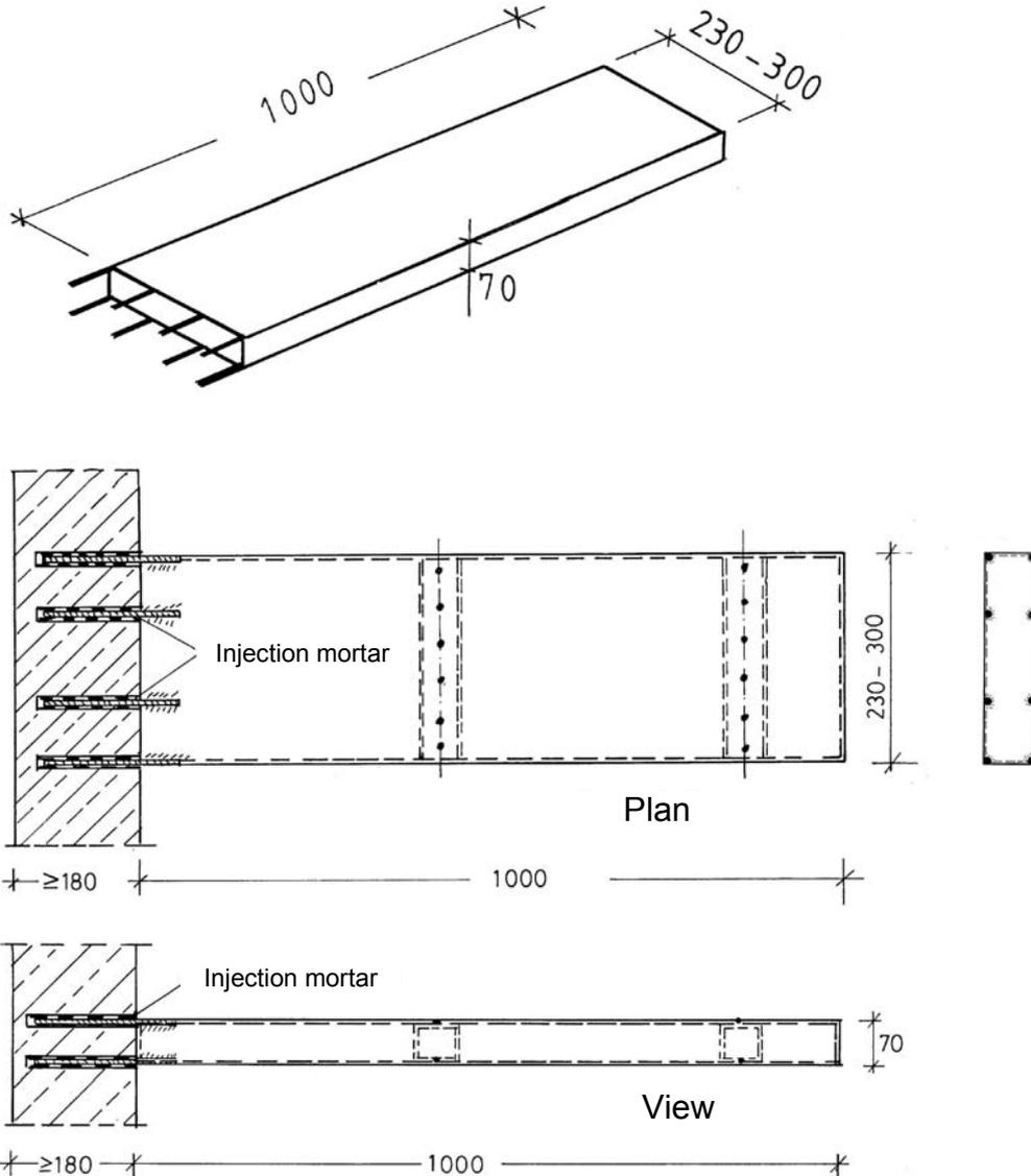
Dimensions in mm, more details (geometry, joints etc.) according to technical documentation
