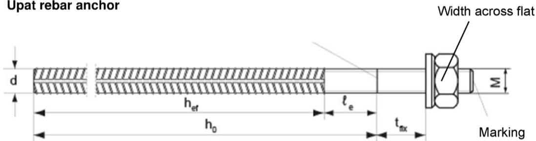
Marking: Upat rebar anchor; FRA (for stainless steel)
