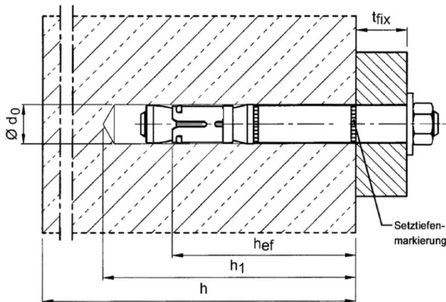
Würth Hochleistungsanker W-HAZ/S, W-HAZ/A4
