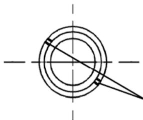
additional marking on end-face for M8x40 and M10x40
