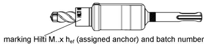
marking Hilti M..x  $h_{ef}$  (assigned anchor) and batch number
