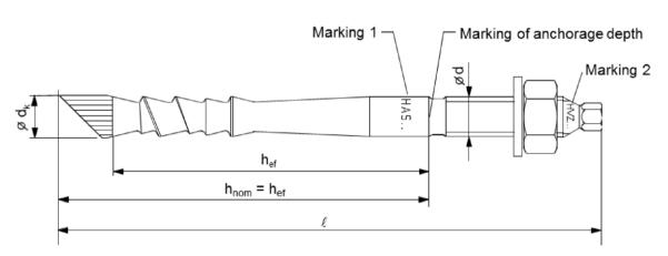
Marking 1: anchor type HAS-(E-)TZ / HAS-(E-)RTZ / HAS-(E-)HCR-TZ
