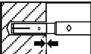
Shoulder of setting tool must fit on anchor rim.
