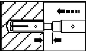
Drive in cone by using setting tool.
