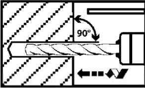
Drill hole perpendicular to concrete surface.
