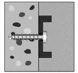
Complete verification: head supported to fixture and embedment depth h<sub>nom</sub>
