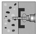
Installation e.g. by hand or with impact screw driver
