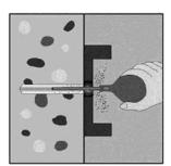
Removal of drill dust Installation e.g. blowing e.g. by hand
