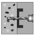
$\begin{array}{l} Drilling \\ Drill \ diameter \\ d_0 \ and \ drilling \ depth \ h_1 \\ have \ to \ be \ kept \end{array}$
