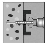
Installation e.g. by hand or with impact screw driver
