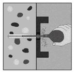
Removal of drill dust e.g. blowing
