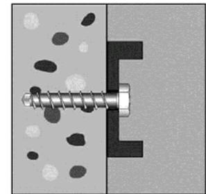
**Complete verification:** head supported to fixture and embedment depth  $h_{nom}$
