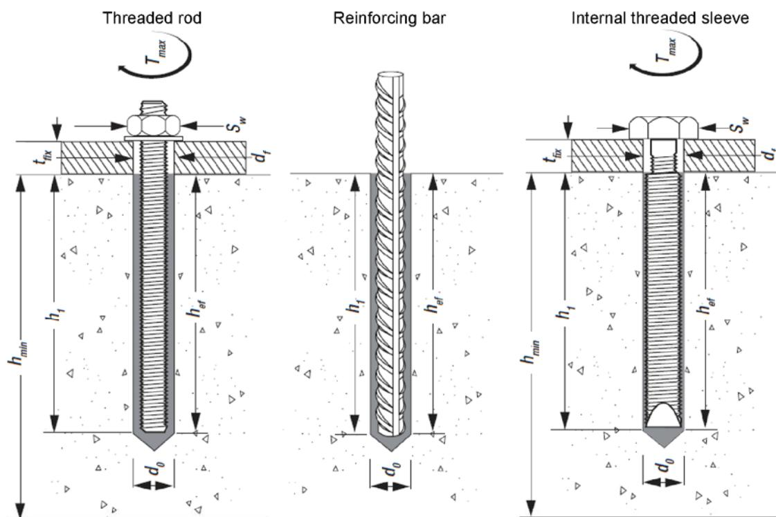
POWERS AC100-PRO Injection resin with anchor rod for concrete
