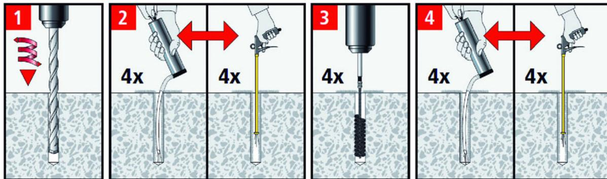
1. Drill with hammer drill a hole into the base material to the size and embedment depth required by the selected anchor (Table B1, Table B2 or Table B3).
