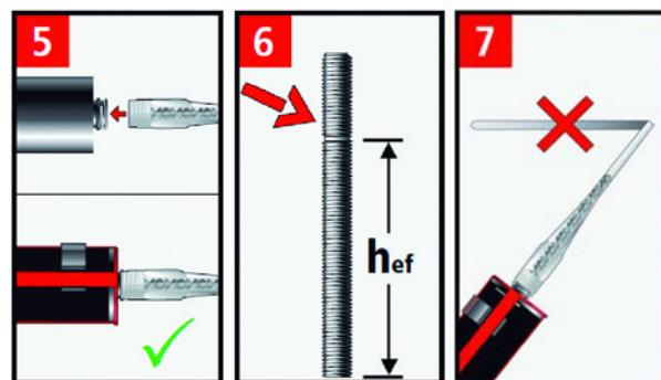
5. Attach a supplied static-mixing nozzle to the cartridge and load the cartridge into the correct dispensing tool. Cut off the foil tube clip before use.
