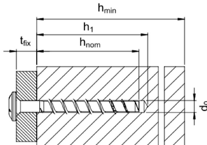
TOGE concrete screw TSM B, BC, BS, BSH
