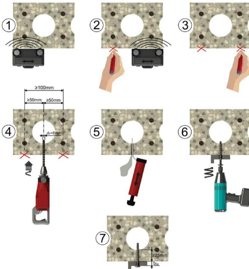
**TOGE concrete screw TSM B, BC, BS, BSH**
