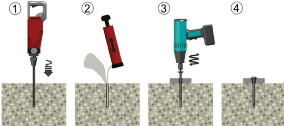
**Installation instructions for anchorages in prestressed hollow slabs**
