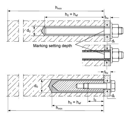
fischer threaded rod pre-positioned anchorage
