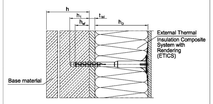
Legend:  $h_D$  = thickness of insulation material
