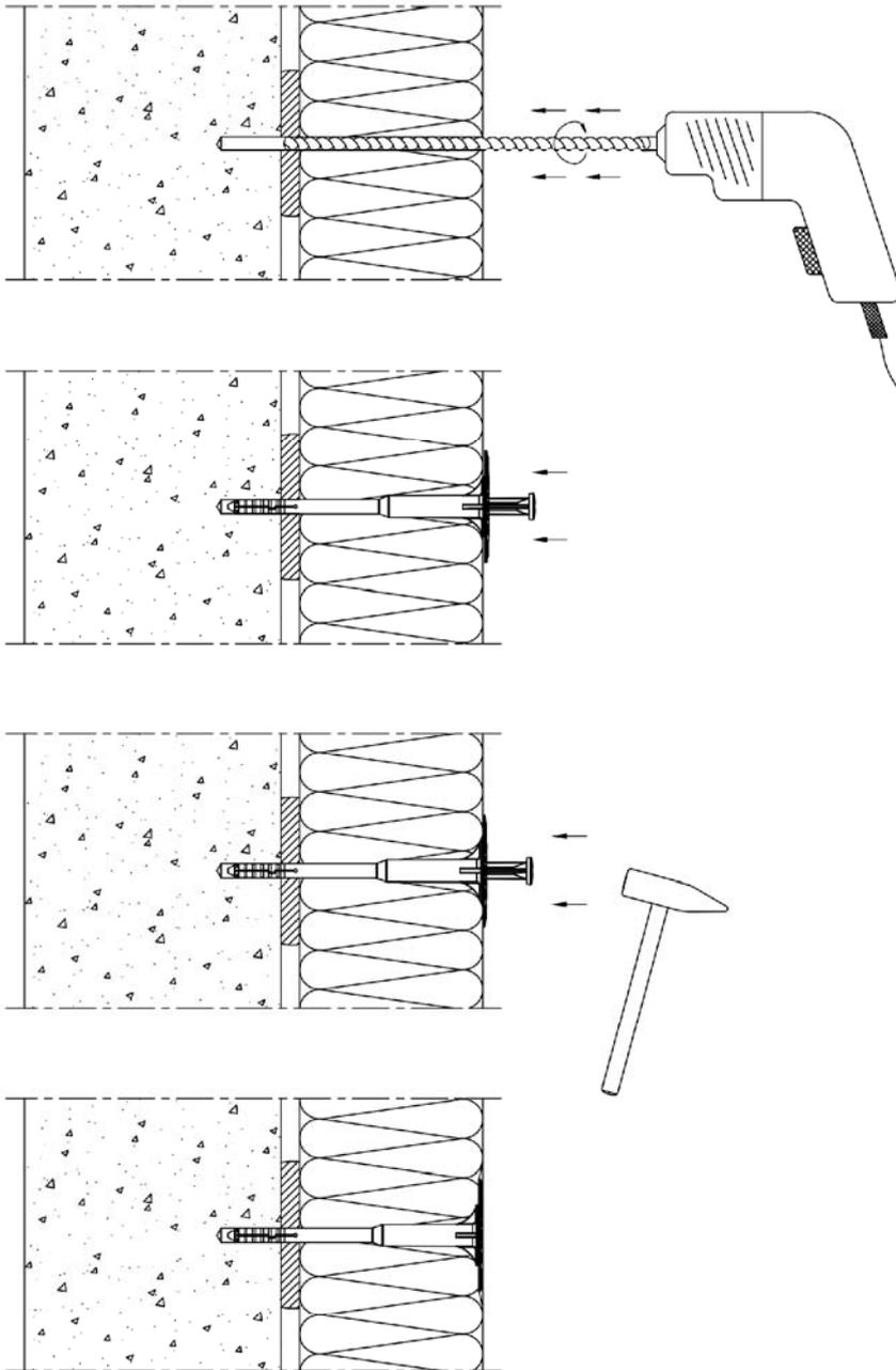
Drill the hole perpendicular to the substrate surface.
