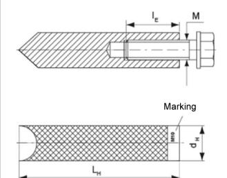
Marking: anchor size e.g.: M10 Stainless steel in addition A4 e.g.: M10 A4 High corrosion-resistant steel in addition C e.g.: M10 C
