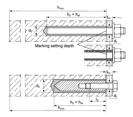
Threaded rod prepositioned anchorage
