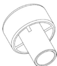
Retaining washer for overhead or horizontal installation
