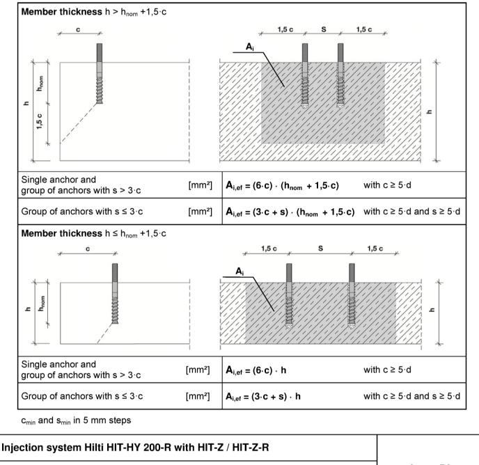
Installation parameters: member thickness, spacing and edge distances
