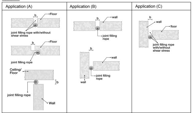
For the number of layers and the arrangement of the joint filling rope
