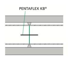
PENTAFLEX FTS – for controlled crack joints in pre-cast elements
