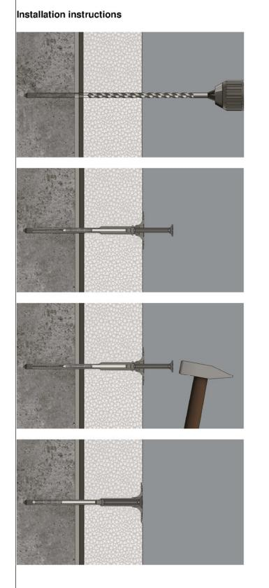
Drill the hole perpendicular to the substrate surface. Clean the drill hole 3x.
