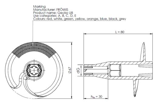
dG = 8 mm (after perforating with the special drill bit)
