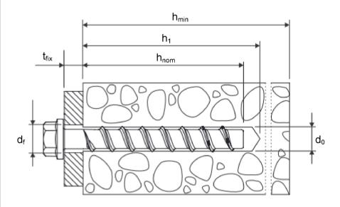
do=nominal drill bit diameterh\_{nom}=nominal anchorage depthh\_1=depth of the drill hole
