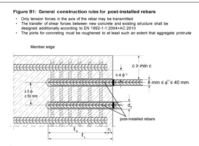
$^{1)}$  If the clear distance between lapped bars exceeds 4  $\phi$  then the lap length shall be increased by the difference between the clear bar distance and 4  $\phi$
